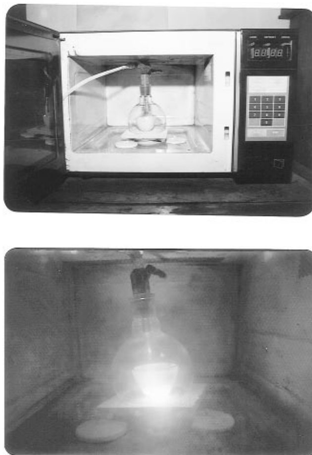
Figure 1. (a, top) Glass reaction chamber used for the containment of necessary atmosphere inside the microwave oven and (b, bottom) the intense glow of the ( TiO_2 + C ) mixture observed within a few minutes of microwave exposure.
